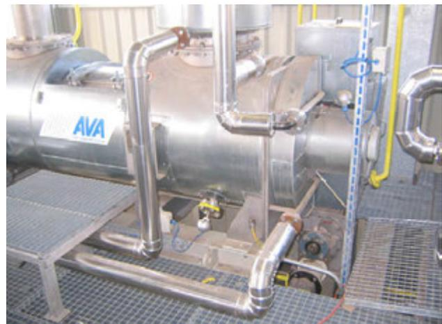
For a continuous drying process, the horizontal shovel dryer HTK-T is used. In a slight underpressure atmosphere, the conveyed salt-solvent mixture is dried and separated from the methanol.
